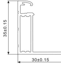
**Dimension of PV Modules** Unit: mm
